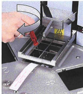
Figure 27 Refitting the transport lock of the heating block (B)
